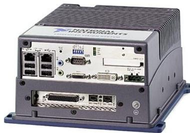
Figure 1: Embedded Vision System (EVS). There are several ports for Ethernet, a display output, USB storage, as well as IEEE1394 ports for cameras
